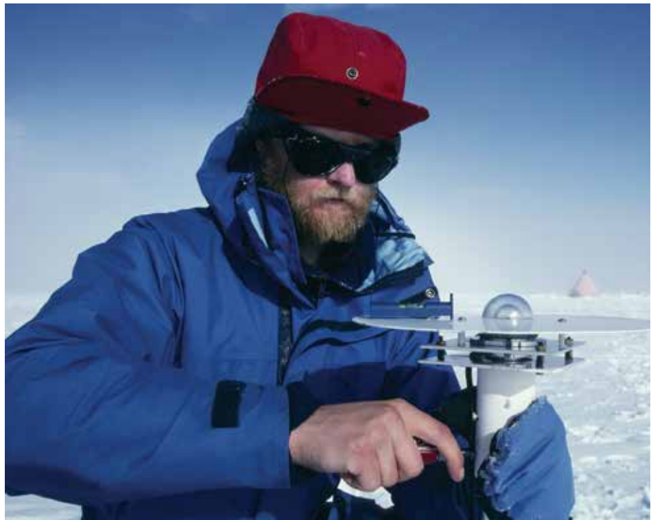
A researcher in Antarctica sets up a recorder that measures the duration of sunlight.
