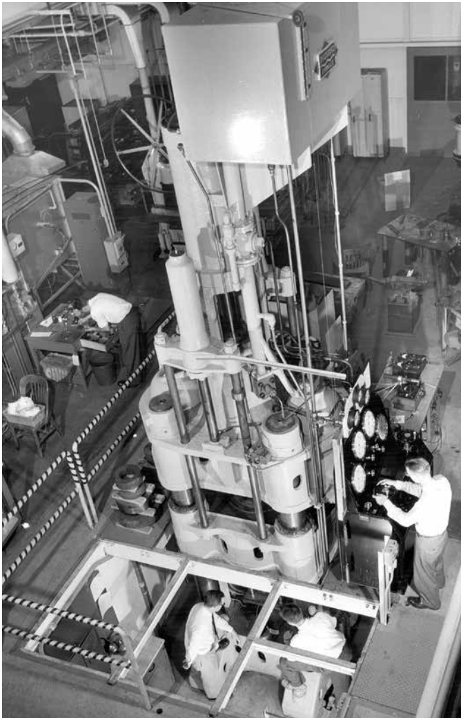
In the 1950s, GE scientists used this machine (in the center of the photo) to create the high pressure and temperature needed to make small commercial diamonds.
